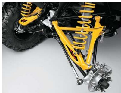
Torsional Trailing A-arms (TTA) independent rear suspension
